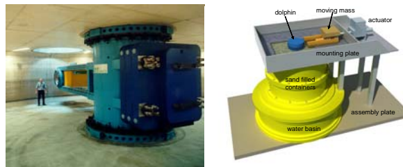
Figure 10. Geo-centrifugal testing equipment and device (GeoDelft)
