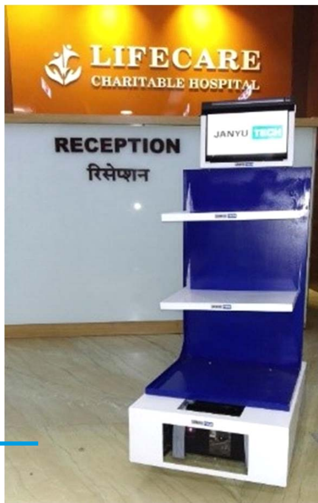
Robotic trolley to supply medicines, food, clothing in isolated wards
