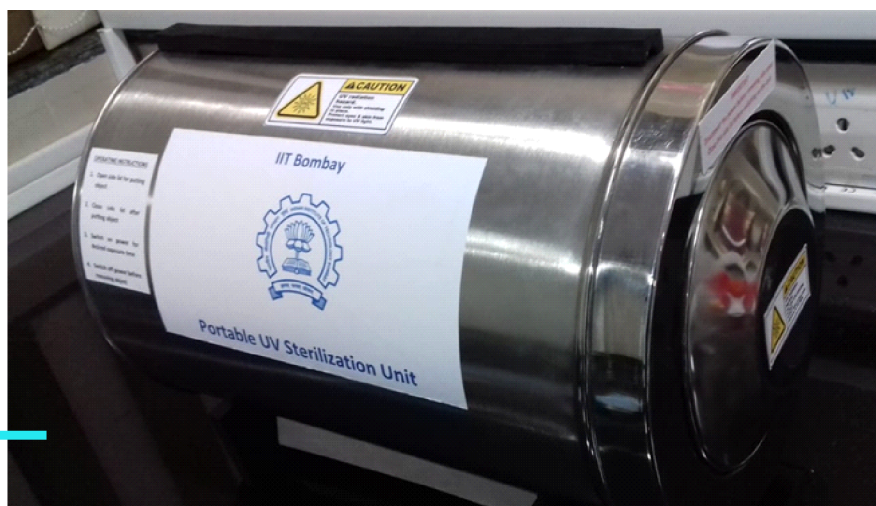
A portable UV sanitizer made to sterilize small items
