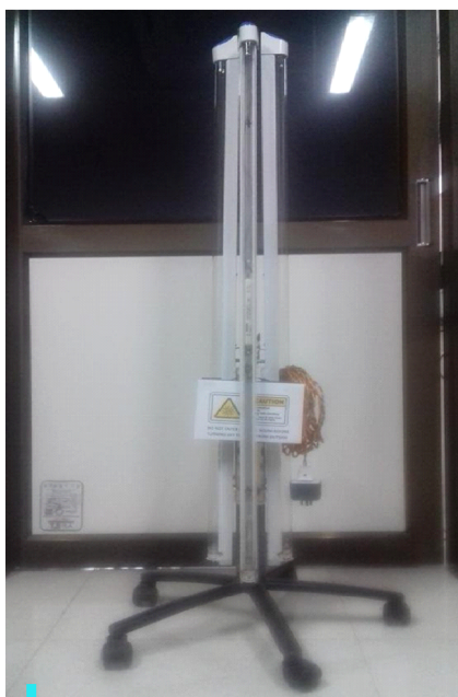
UV sanitizer can be easily transported from one place to another to disinfect virus
