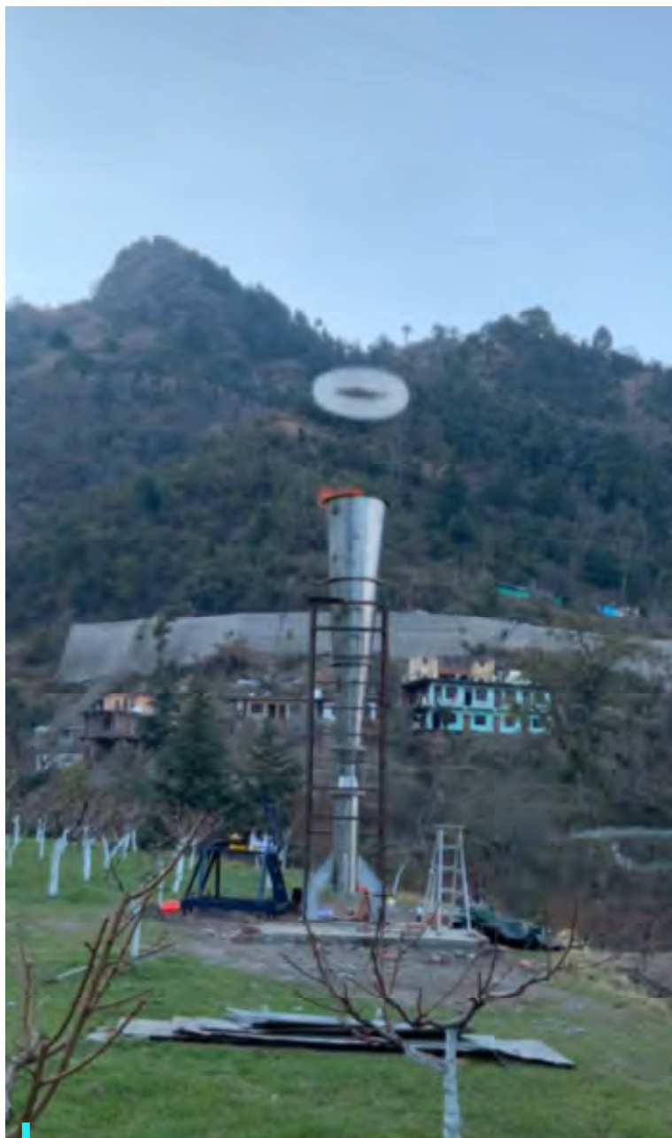
Anti-hail cannon, indigenously built by IIT Bombay, works with LPG fuel and is cost-effective
