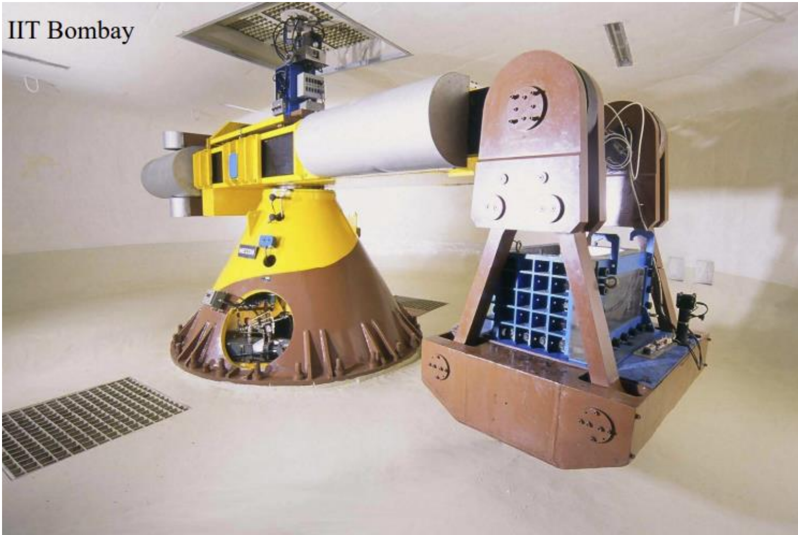
Figure 2c View of the 4.5 m radius large beam centrifuge facility
