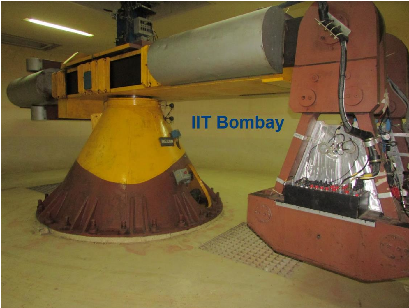
Figure 2a Perspective view of 4.5 m radius large beam centrifuge facility at IIT Bombay
